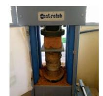
Figure 8: Crushing test of a compressed brick
