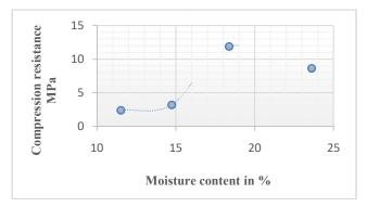
Figure 9: Curve of compressive strength as a function of water content
