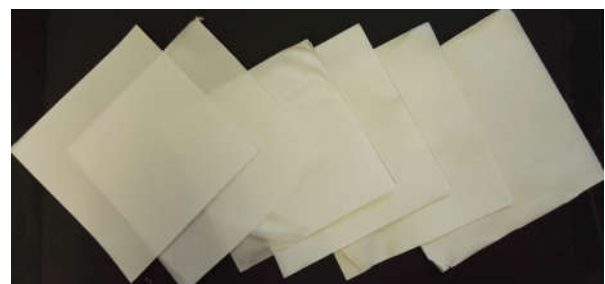
Figure 2: Spray Coated Nanocomposites prepared via spraying cellulose nanofiber -MMT produced from spraying of CNF -Cloisite Na ++ suspension on the stainless-steel plate. The size of cellulose nanofiber composite is 220 mm x 220 mm and thickness vary from ~81.7µm to 135.8µm. The basis weight of the film varies from ~70 g/m 2 to ~100g/m 2 .
