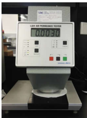
Figure 6: Measurement of Air permeance of spray coated nanocomposite
