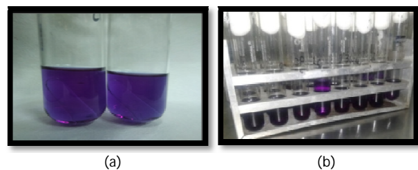
Figure 2: (a) Test tubes with MacConkey Broth; (b) Set of test tubes with MacConkey Broth and sample in it before incubation.
