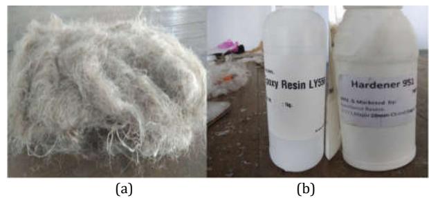
Figure 3: (a) Jute fiber, (b) Epoxy resin LY556 and Hardener
