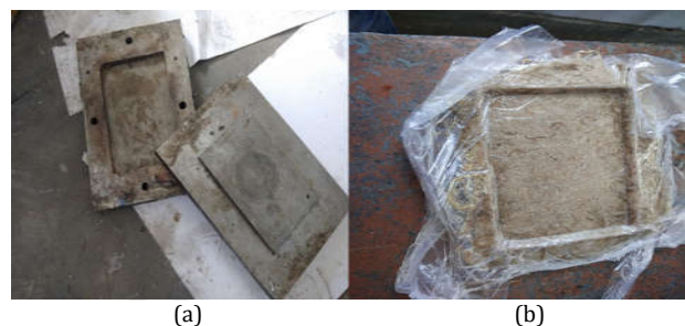
Figure 4: (a) Mild Steel Mould, (b) Mould after filling fiber with epoxy
