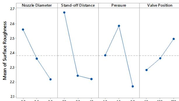
**Figure 3:** Main effect plots for surface roughness considering water vapour related parameters: Effect of nozzle diameter, stand-off distance, pressure and valve position
