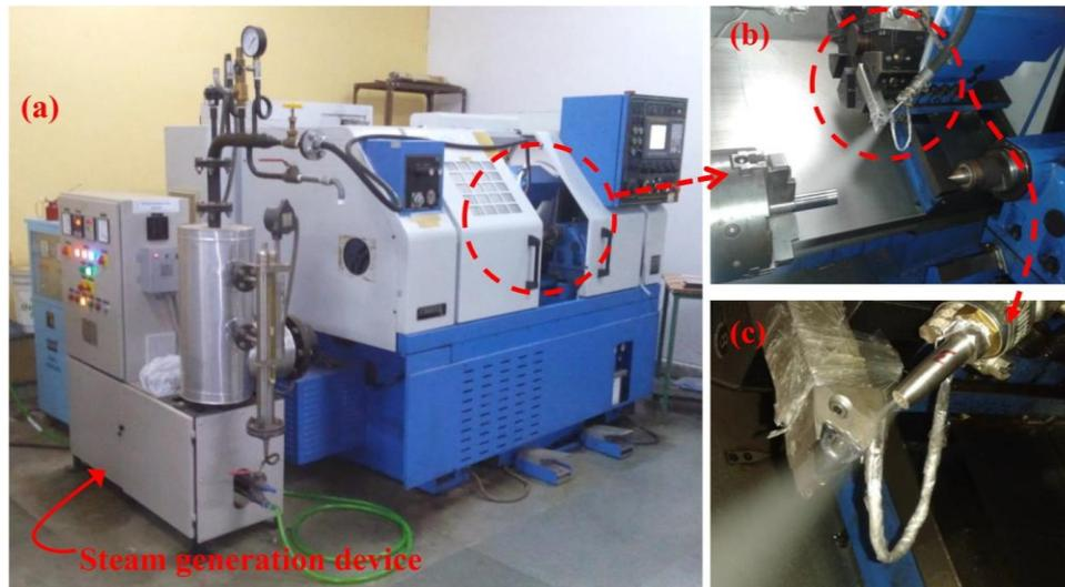
**Figure 1:** (a) Steam Generation Device and supply of water vapour to machining zone (CNC turning lathe) through hose; (b) Water vapour jet directed into machining zone through nozzle held in fixture, and (c) Water vapour jet flow visual close-up view
