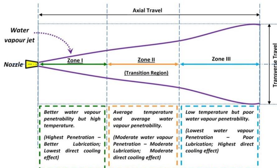
**Figure 2:** Basic characteristics of a water vapour jet flow [30]
