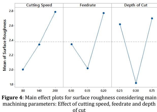
**Figure 4:** Main effect plots for surface roughness considering main machining parameters: Effect of cutting speed, feedrate and depth of cut
