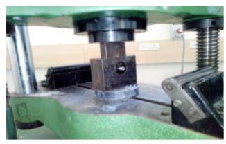
Figure 6: Shear test on UTM
