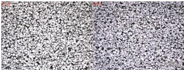
Figure 2: Optical micrographs of DSIT at deformation temperature (a) 850 °C and (b) 770 °C for 0.14C-0.64Mn steel [23]
