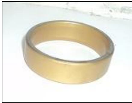
Figure 1: Bearing outer race coated with TiN
