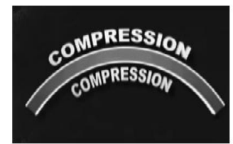
Figure 15B: After shot peening
