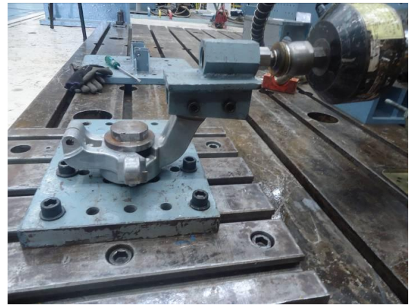
Figure 17: Rig level setup for durability test
