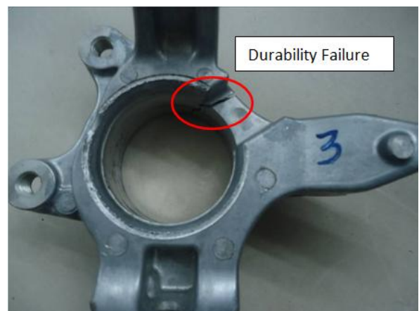
Figure 18: Steering knuckle failure post durability test
