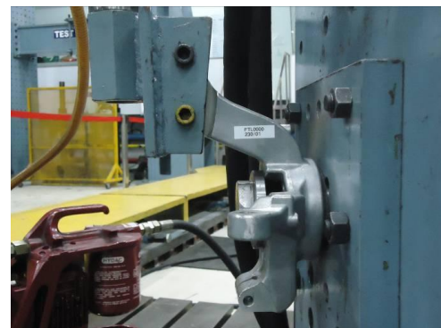
Figure 4: Fixture setup for static strength test
