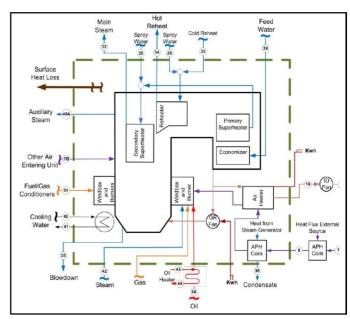
Figure 1: Steam boiler control volume according to PTC 4 standard [8].
