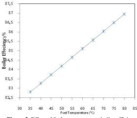
Figure 2: Effect of fuel temperature on boiler efficiency
