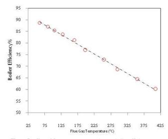
Figure 7: Effect of flue gas temperature drop on boiler efficiency
