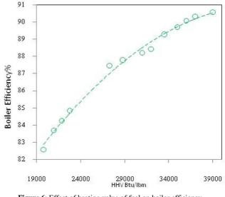
Figure 6: Effect of heating value of fuel on boiler efficiency
