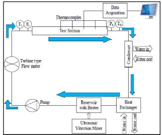
Figure 1: Schematic of Experimental Setup
