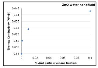
Figure 3: Thermal conductivity enhancement of ZnO-Water nanofluid.
