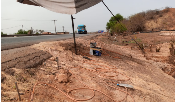
Figure 4: Implementation of an electrical resistivity profile downstream of the insertion pit
